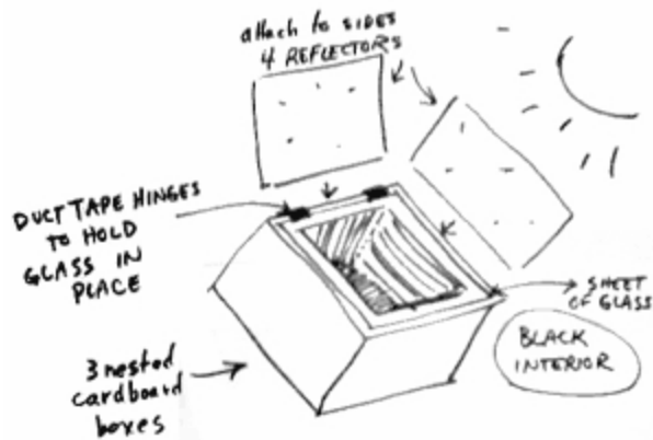
A solar oven design made with cardboard boxes, aluminum foil, and a piece of window glass. Interior of the box is flat black paint.
